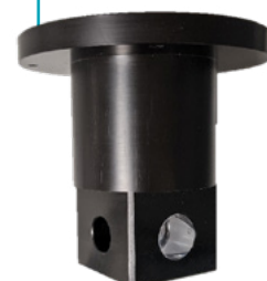
Dry check tool Manual use two positions for 2 steps : • Dark level • Low scattering level
