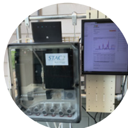
6 STAC2 • UV Online Analyzer for COD BOD TOC TSS NO 3
