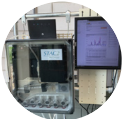
UV Online Analyzer for COD BOD TOC TSS NO 3
