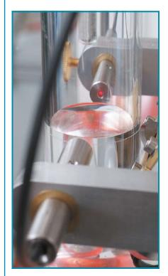
Meniscus is determined automatically at the exact lowest level by a laser beam.
