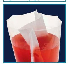
Bags with full (page) filter divides in 2 equal compartments. Solid sample remains in it's side, while the liquid phase moves to the other side.
