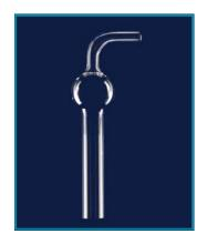
Manufactured from heat resistant, durable borosilicate glass according to DIN 12610 standard with a ball and connection tube.
