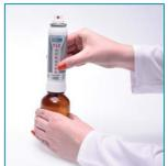
**Mounting:** Attach TLC sprayer to the bottle by turning anti-clockwise. Never shake the sprayer during mounting.
