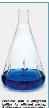
Baffles create a turbulent flow, enlarge gas exchange surface and increase oxygen intake.
