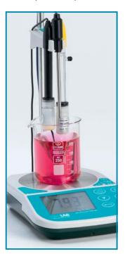
Table top meters have a special platform with a magnetic stirrer which enables fast and accurate measurements and results.
