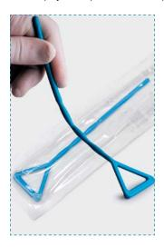
Handle flexes slightly under pressure allowing the triangular head for perfect, evenly distributed and uniform pressure on the agar surface.
