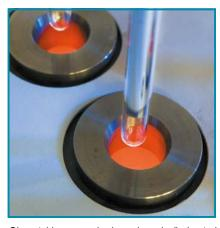
Glass tubings are slowly and gradually heated up to half-melting level. Then they are shrinked around steel rods with precise diameter.
