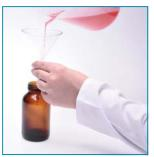
**Filling:** Pour the TLC reagent into the bottle. Never fill above the shoulder line.
