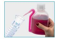
Dispensing tip provides extra fine stream. The tip of the delivery tube can be cut in order to increase the liquid flow rate.
