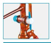
All automatic burettes are featured with an intermediate PTFE stopcock for reliable, fast and accurate measurement.
