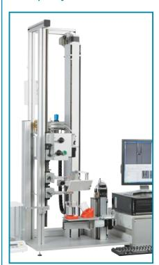
Steps such as filling the water, finding the meniscus line and controlling the volume are done automatically.
