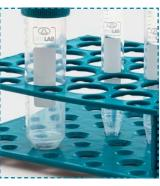
Holes at the bottom plate guarantee firm hold of tubes in their position.
