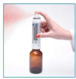
**Spraying:** Start spraying with the sprayer and release the button while the sprayer is still moving at the end of the TLC plate to avoid reagent loss. For best performance a spraying angle between 90° and 45° is required.
