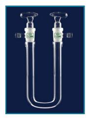
Manufactured from heat resistant, durable borosilicate glass according to DIN 12616 standard with a U form and featured with a stopcock.
