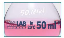
Net volume with 0,001 ml presicion is engraved on the body of calibrated density bottles.
