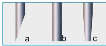
**"A" type needles** are designed for optimum penetration with 17° bevel. Also minimizes the necessary piercing force and diameter of injection channel.
