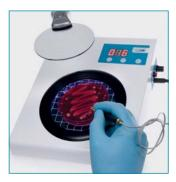
Marking is done by a "felt pin pen" which is connected to the system by cable.
