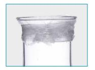
Offers extremely good stretching, and adhesion characteristics. Perfect tool for sealing and wrapping of various labware.
