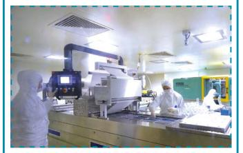
ISO LAB sterile production plants are well equipped clean rooms with **HEPA filters** and positive pressure areas which are supplied with air locked doors.
